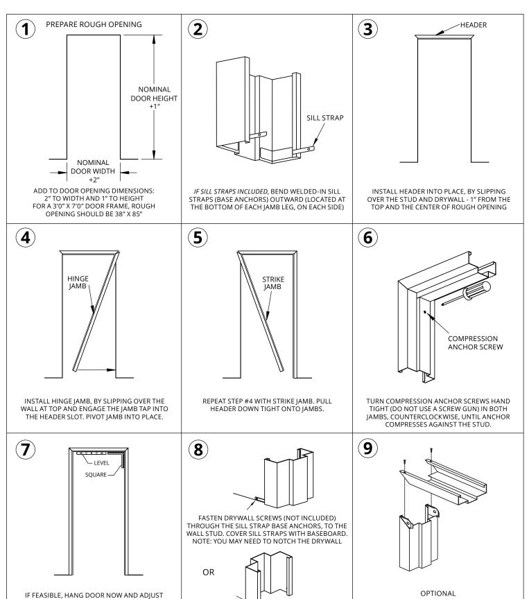
FASTEN SCREWS TO THE WALL STUD, THROUGH HOLES
