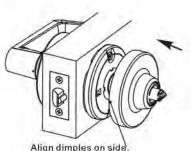
**2E:**Remove inside lever and install inside rose, make sure inside rose is fully snapped in.
