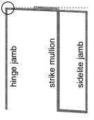
If the level indicates that the hinge jamb side is higher than the strike jamb, fasten one screw in the header over the hinge jamb. Align the corner of the hinge jamb with the corner of the header and fasten at an upward angle at the top of the hinge jamb to ensure that it is snug to the header.
