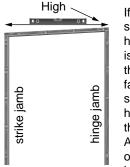
If the level shows that the hinge jamb side is higher than the strike jamb, fasten one screw in the header above the hinge jamb. Align the corner of the hinge jamb with the
