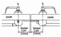
Rim exit device and surface vertical rod exit device combination
