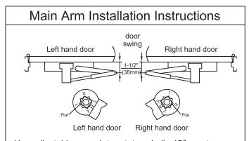
Use adjustable wrench to rotate spindle 45° counterclockwise for right hand door or clockwise for left hand door. Place main arm on spindle so that the "R"(Right hand door) or "L"(Left hand door) lines up with the spindle flat. Secure main arm and spindle by tightening spindle bolt.
