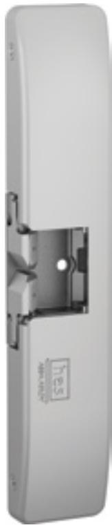
The 9500 series is a 3 hour fire-rated, surface mounted electric strike designed to accommodate rim exit devices with a 3/4" throw Pullman latchbolt. All components are completely encased within its 3/4" thick stainless steel housing, so no cutting on the frame is required for installation. Simply place the electric strike on the surface of the frame, align it with the exit latchbolt and install. Adjustments have never been easier as the base is now separate from the cover.
