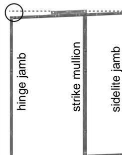
If the level indicates that the **hinge jamb is lower than the strike jamb**, lift the header until it is level and fasten one screw in the header over the hinge jamb. Lift the hinge jamb tight to the header. Align the corner of the hinge jamb with the corner of the header and fasten at an upward angle at the top of the hinge jamb to ensure that it is snug to the header.
