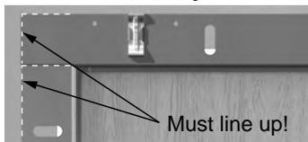
16. Replace the strike mullion and fasten to the mullion bracket on the header on both sides.
