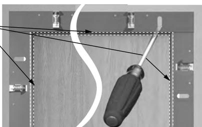
12. Hang the door. Close the door in order to align it with the frame. Begin with the header using a screwdriver through the alignment slot closest to the strike mullion. Create an equal gap between the door and frame. Fasten the header above the strike mullion and the remainder of the header at every clip on the door side only.
