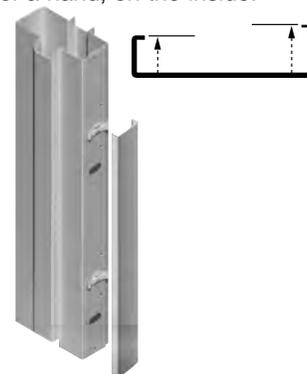
f. On the horizontal mullion casing, make sure its longer side faces down.
