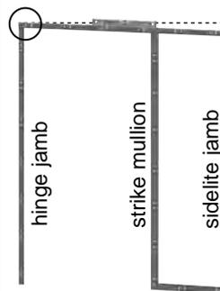
If the level indicates that the **hinge jamb side is higher than the strike jamb**, fasten one screw in the header over the hinge jamb. Align the corner of the hinge jamb with the corner of the header and fasten at an upward angle at the top of the hinge jamb to ensure that it is snug to the header.
