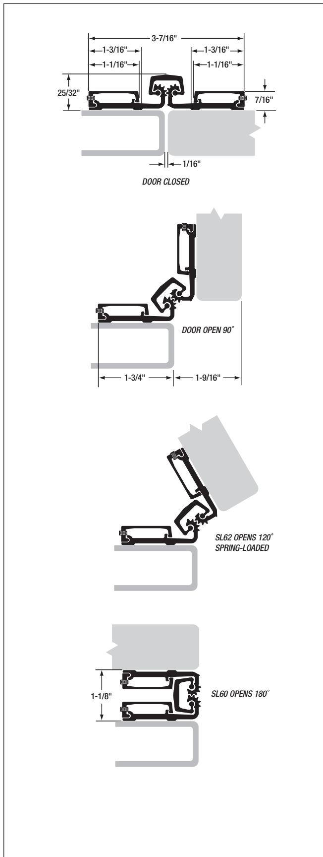
**MATERIAL:** Extruded 6063 T6 aluminum alloy with self-lubricating polyester thrust bearings.
