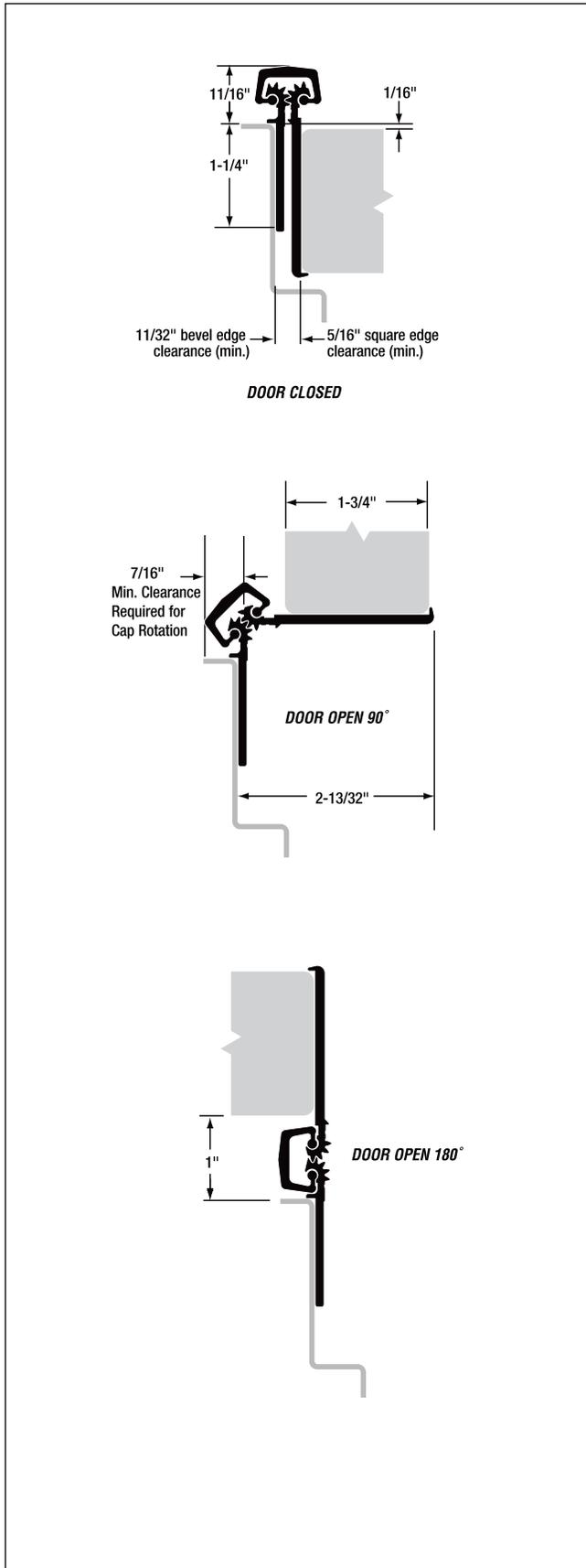
**MATERIAL:** Extruded 6063 T6 aluminum alloy with self-lubricating polyester thrust bearings.
