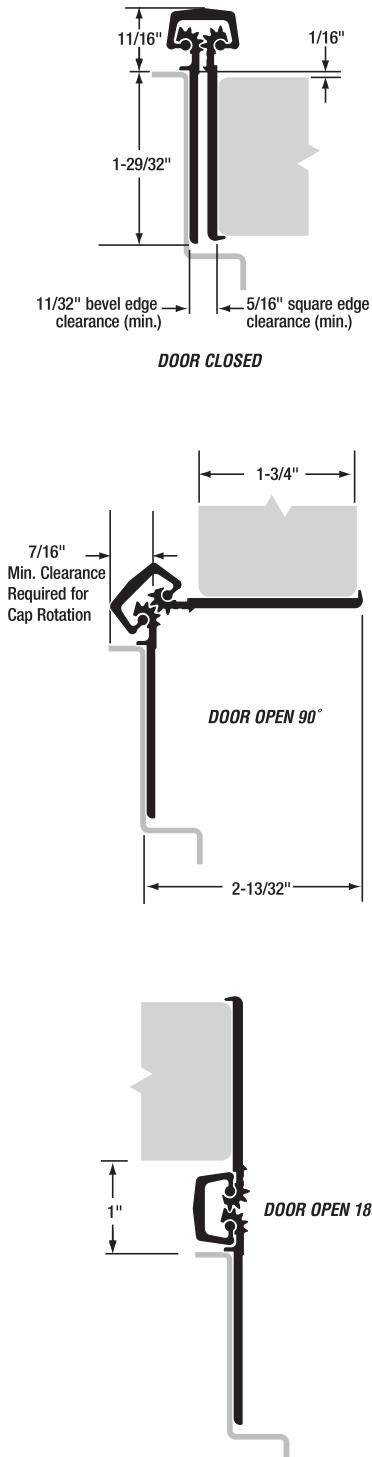
**MATERIAL:** Extruded 6063 T6 aluminum alloy with self-lubricating polyester thrust bearings.
