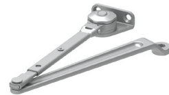
4030-3049L Hold Open Long Arm (HLONG) • Non-handed • Includes long head and tube, 4030-3048L for top jamb mount with deep reveals • Optional
