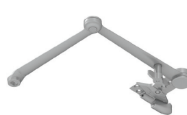
4110-3049SCNS Spring Hold open Cush-n-Stop Arm (SHCUSH) • Non-handed • For abusive applications features solid forged steel main arm and forearm with spring loaded stop in the soffit shoe • Handle controls hold open function • Optional
