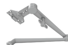
4030-3049SCNS Spring Hold Open Cush-n-Stop Arm (SHCUSH) • Non-handed • For abusive applications • Features solid forged steel main arm and forearm with spring loaded stop in the soffit shoe • Handle controls hold open function • Optional
