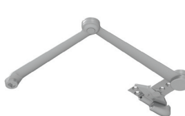
4110-3077SCNS Spring Cush-n-Stop Arm (SCUSH) • Non-handed • For abusive applications features solid forged steel main arm and forearm with spring loaded stop in the soffit shoe • Optional
