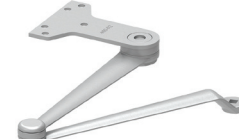
4030-3049EDA Hold Open Extra Duty Arm (HEDA) • Handed • Arm, provides hold open function adjustable at shoe • Optional
