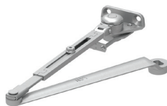
4110-3049FL Fusible Link Arm (FL) • Handed • Releases hold-open function adjustable at shoe when exposed to temperatures above 165° F • Optional
