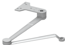
4110-3077EDA/62G Extra Duty Arm (EDA) • Non-handed • Features forged, solid steel main and forearm for potentially abusive installations • Optional 4110-62G thick hub shoe for blade stop clearance
