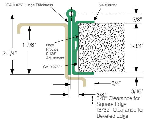
\* Adjusta-Stud allows up to 3/8" width adjustment which ensures proper alignment and easy installation. Adjusta-Stud also makes it possible for future adjustments of the door on the frame through repositioning.
