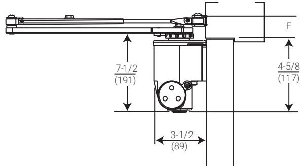
Body mounting holes are spaced 4-1/8" (105mm) horizontally and 1-3/8" (76mm) vertically.
