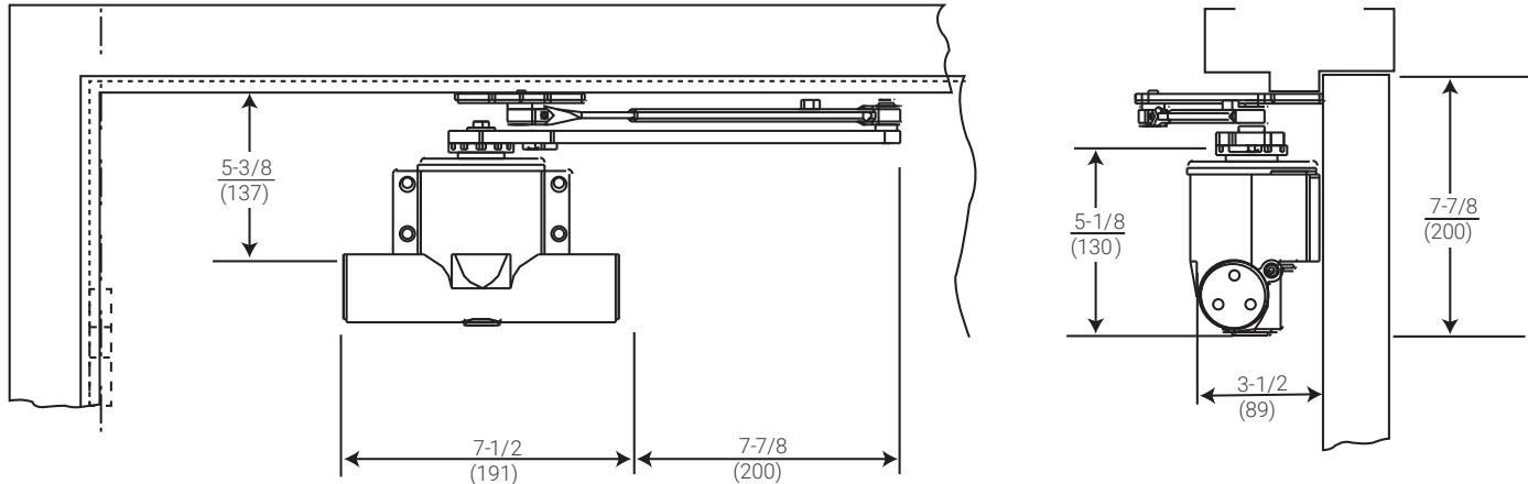
Body mounting holes are spaced 4-1/8" (105mm) horizontally and 1-3/8" (76mm) vertically.
