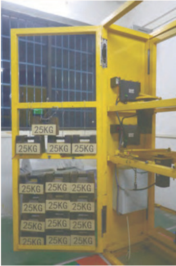
790 lbs (360kg) Load-Bearing Test
