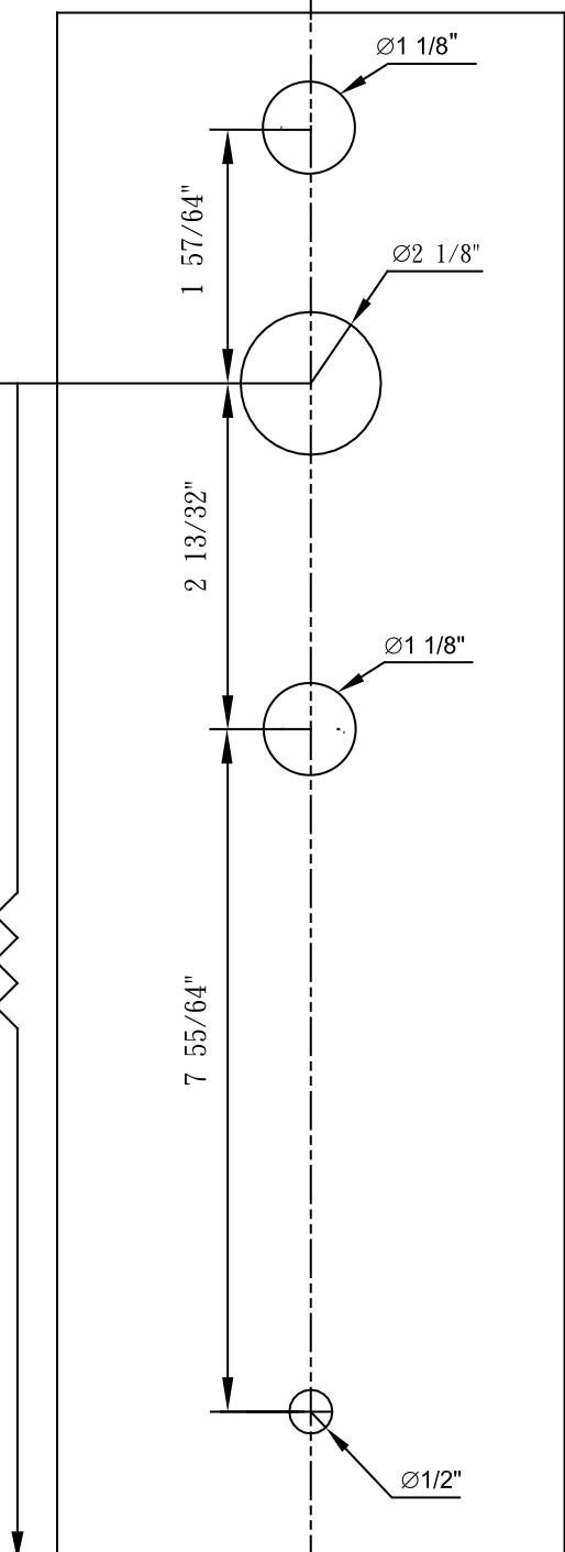
Note: If 2P-02DT is being used then 2 1/8" hole, Rim cylinder and cylinder sleeve are not used.
