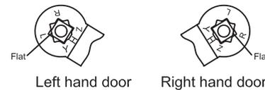
Use adjustable wrench to rotate spindle 45° counter-clockwise for right hand door or clockwise for left hand door. Place main arm on spindle so that the "R"(Right hand door) or "L"(Left hand door) lines up with the spindle flat. Secure main arm and spindle by tightening spindle bolt.
