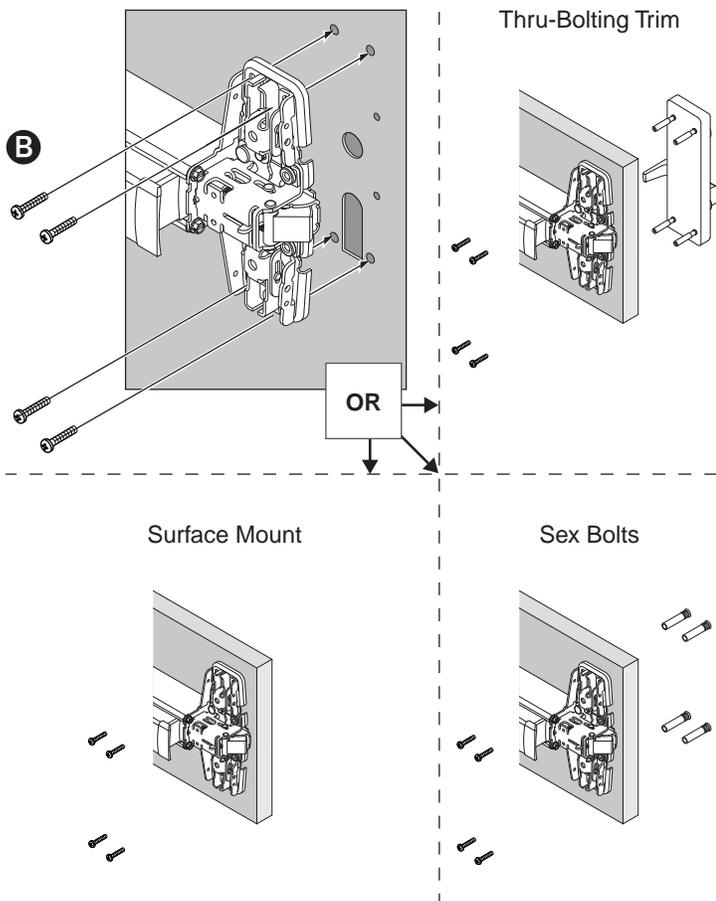
**13** Install end cap bracket and end cap.
