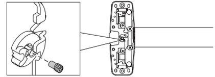
With the NL drive screw removed, key locks and unlocks lever, knob, or thumb piece. For the trims listed below, **REMOVE** NL drive screw.
