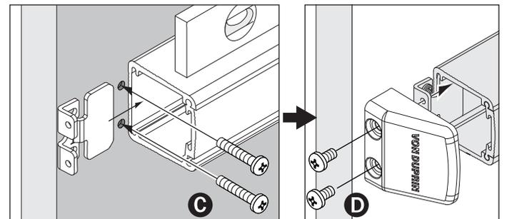
**14** Install required support screws and center case cover.
