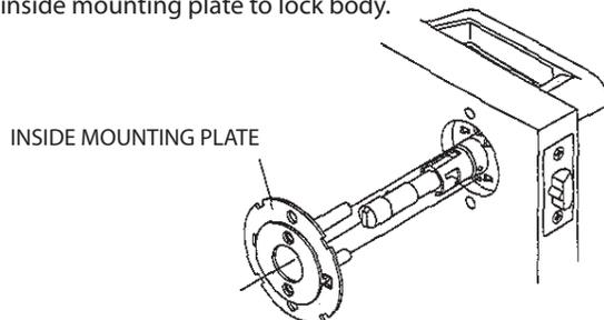
B. Press inside rose liner onto mounting plate and tighten mounting screws securely.
